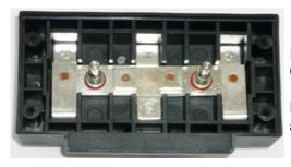
If contact plates are burned or corroded, clean with fine sand paper. Contact surface are where the metal plates have contact.
